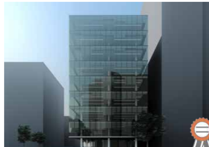
From top to bottom: Southeast, south and east perspectives of the double glazing option. The DGU performance has been judged as poor based on the non-uniformity of occupant-controlled blinds.
